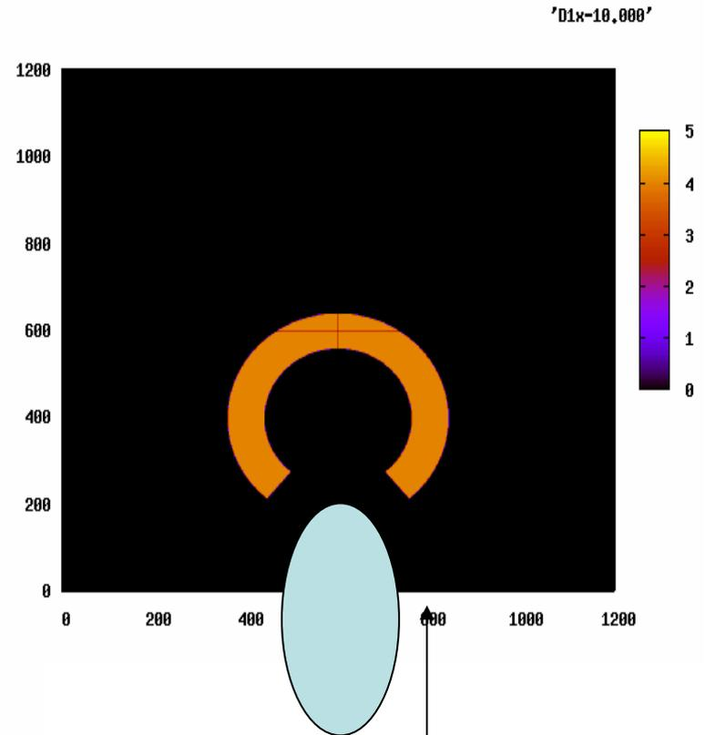
The shell is heated by laser from inside,
